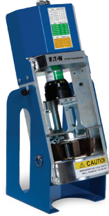
ET1187 Crimp Machine shown with base frame. (Part number: ET1187-001 Kit, includes ET1187C-0017 bench top stand).
